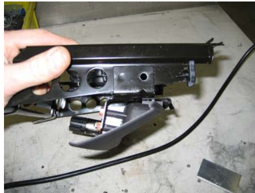
Drill out spot-welds that hold the power point bracket to the frame. This needs to be removed in order for the console to slide into the rail
